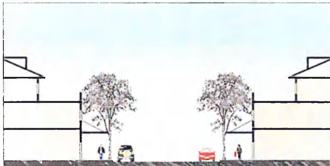
Proposed street section for Monash Road with building step back at third storey
